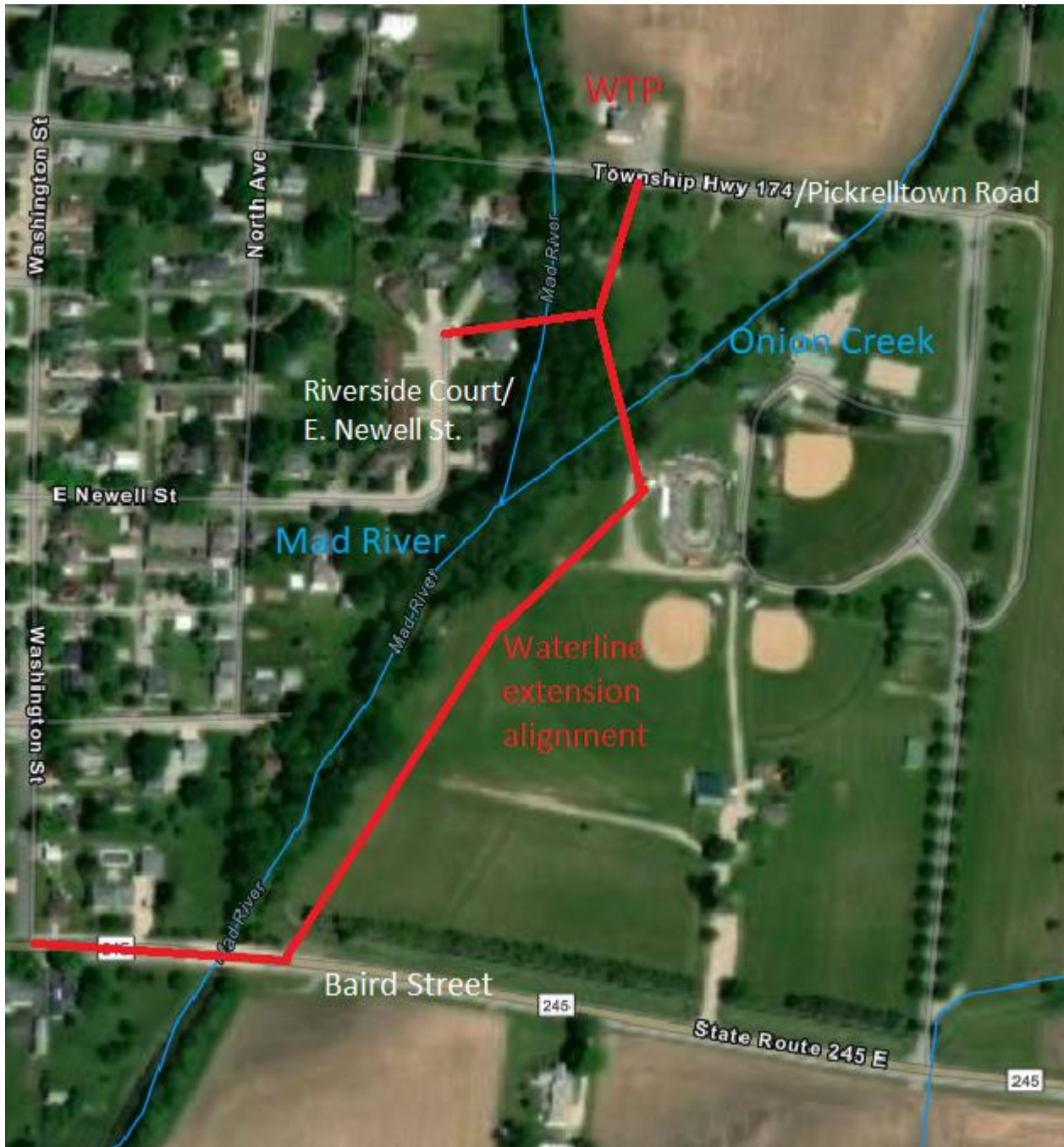
Figure 4. Map of waterline alignments part 2 and 3, crossing under the Mad River and Onion creek.
